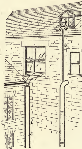
Fig. 604. A, soil pipe communicating with sewer and opening just below bedroom window. B, Ventilator of soil pipe discharging close to the attic window.
